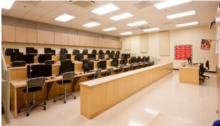
Red Pump Elementary School, Bel Air, MD (Design by GWWO) Tiered seating allows the students' computer screens to be easily seen from one location by the instructor. Half walls can be used as a secondary work surface when students face the teaching wall.
