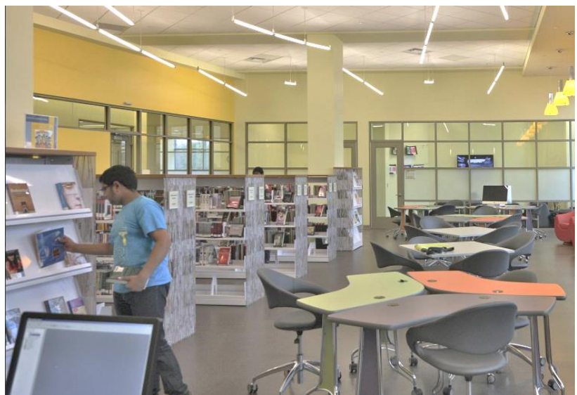
Gum Spring Library; Loudoun County, Virginia (Design by Grimm + Parker Architects; Photo by: Ken Wyner) The lighting fixtures deliberately do not define different functional areas to allow the maximum flexibility in how the space is arranged.
