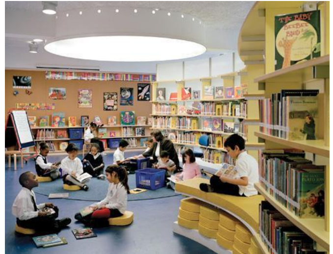
FINISHES: Seamless vinyl floor, a cork wall, colorful foam cushions and curvy laminate plywood shelving create a comfy space.
