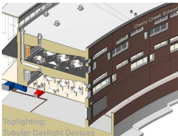
Cherry Creek School, Greenwood Village, Colorado (Design by Hutton Architecture Studio) Diagram of the tubular daylight device system, allowing natural light to penetrate lower floors of a school. Credit? Drawing of tubular daylight device in
